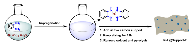
Fig. 2 Preparation of supported nickel nanoparticles by the immobilization and pyrolysis of the Ni-diamine complex on an active carbon support.
